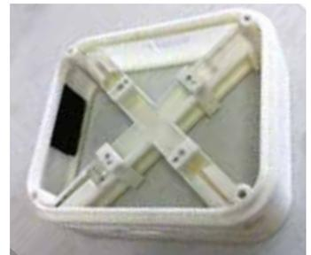
FDM bracket used to the legs of a UAV.
