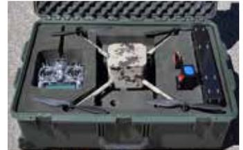
The RDASS 4 fits into a compact case for easy transport and fast deployment.
